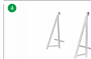
Find the 30*30 square tube also placed under the base beam of the tripod
