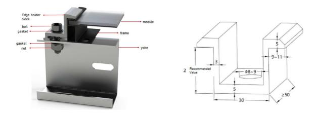
Pressure clamps should not come into contact with the glass surface of the module and must not deform the frame. Be sure to avoid shadowing effect from the pressure clamp.
