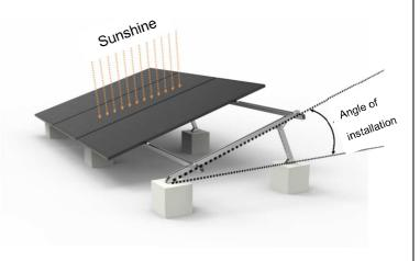
the difference in the total amount of solar radiation absorbed by photovoltaic modules, resulting in the mismatch loss of output power, thus reducing the operating efficiency of the system.
